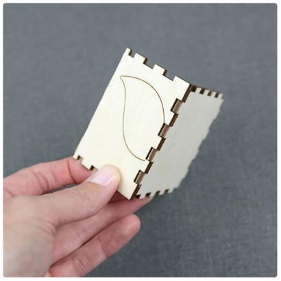
Next, take piece F and attach it to the back of piece J. This creates the back wall of the lower half of the box. The engraved tail detail should be facing outward and visible.
