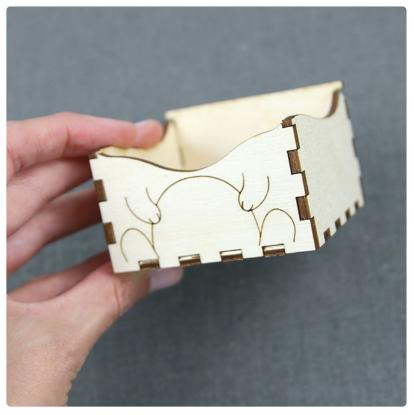
Attach piece H to the front of J so that the engraved details are facing out. This completes the lower half of the box.
