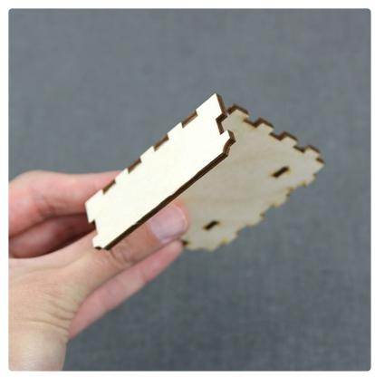
To start, attach piece A to the back of piece E (the side farthest from the two top slots). This creates the back wall of the box lid.
