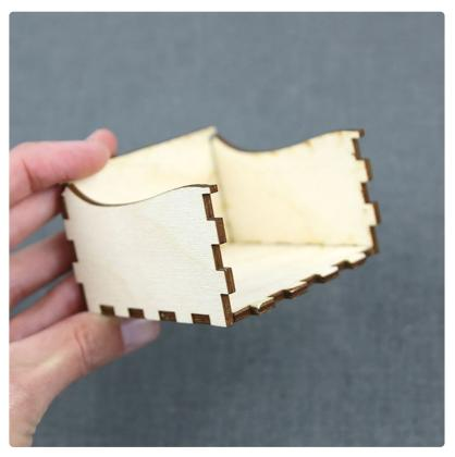
Attach piece G to the side of J so that the highest point of the curve faces the back. Repeat this same step on the other side with piece I.
