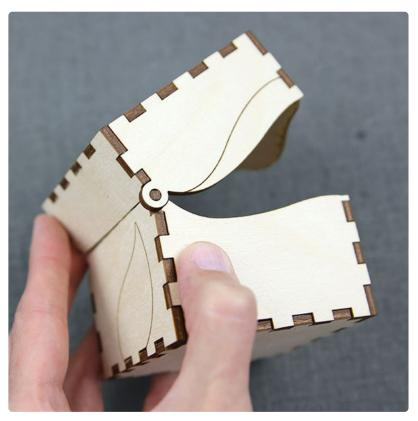
Next, slide the circular hinge piece of piece B over the thin tab at the top of piece F. The hinge element should sit neatly between where both F and G meet at the corner.
