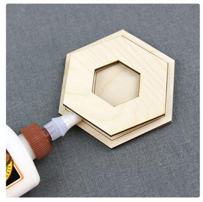
Next, glue piece I to the underside of C/D. Use the scored line as a placement guide.
