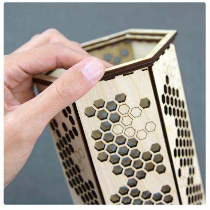
Finally, fit the slots of the assembled box top (from step two) into the tabs of pieces F-1 through F-6 on the box walls.
