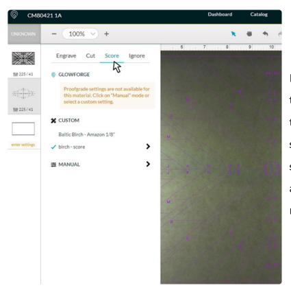
Follow the cutting guide PDF to select the layers and set them to either cutting or scoring in your laser cutting software. Repeat this step until all files are cut. Once complete, remove the masking tape.
