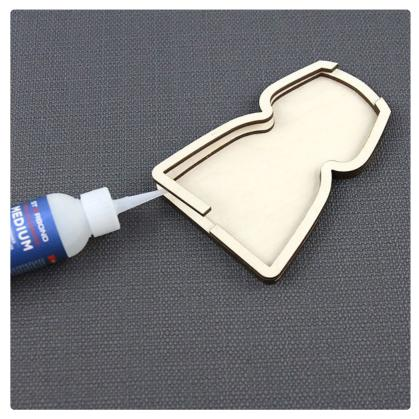
Take a set of spacing layer pieces and, matching the edges of the candyholder, glue them on top of the solid outline layer. All of the spacing layers are cut so that there is a gap at the top.
