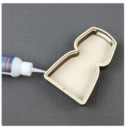
The wood frame layer that holds the acrylic window layer in place may look similar to the thick outline layer and spacing layers, but it will have a thinner edge and be in one piece. Glue this piece on top of the spacing layers, lining up the edges with the sides of the candy holder. This will hold the acrylic window layer in place.
