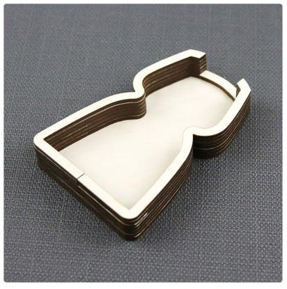
Repeat with the remaining spacing layers. If you want a deeper candyholder, simply cut and glue additional spacing layers.
