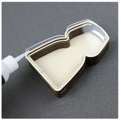
Since the wood frame layer is half the width of the spacing layers, the inner edges of the spacing layer will stick out, creating a ledge. Glue the acrylic window layer onto this space. You don't need much glue for this step, just a few drops around the edges which will be hidden by the top layer.
