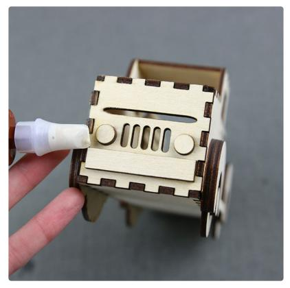
Using the scoring lines as a guide, glue pieces I-1, I-2 and L-1 to piece D.
