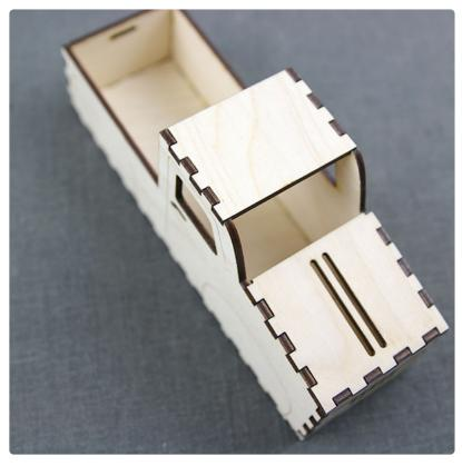
Attach piece B to the top of pieces A-1 and A-2, closing in the top of the truck body.
