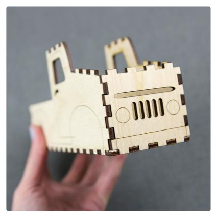
Attach piece D to the remaining side of piece K to form the front of the truck.
