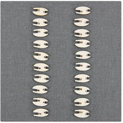
Before beginning wing assembly, it may be helpful to sort the wing joint pieces into two piles, one marked with an R on the bottom for right wing, and the other marked with L on the bottom for the left wing.
