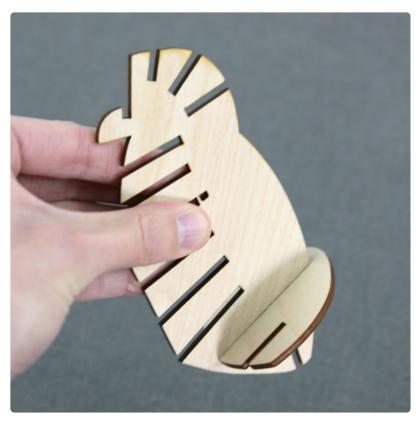
Slide the middle slot of piece D into the lowest horizontal slot on the back piece B.
