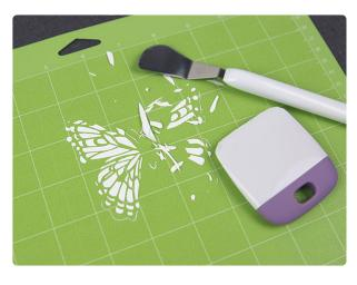
After the design has been removed, there will likely be paper still stuck on the mat. If there are any big pieces remaining that you would like to reuse in the future, flip the mat over and remove them using the same process as was used for the design. If there are small pieces remaining that are going to be recycled or thrown away, simply pick or scrape them off using tools or your fingers.
