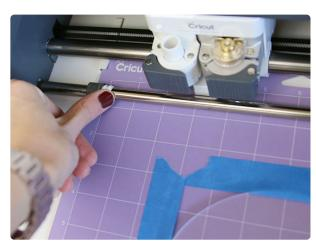
Most cutting machines have little wheels or feet on their roller bar to assist with pulling the mat in and out of the machine. These wheels can damage the acrylic or push it out of place.
