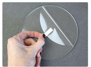
After selecting and purchasing your acrylic and design, it's time to prepare the acrylic for engraving. Most acrylic will come with a protective film on both sides to protect it from dust and scratches.
