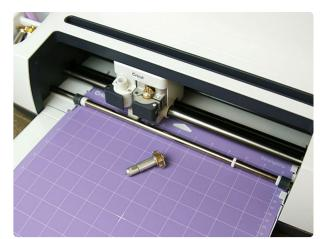
Before purchasing any acrylic, make sure your cutting machine is capable of engraving on acrylic by referencing your company's website or handbook. For example the Cricut Maker has the engraving tip, and the Silhouette Curio has the stippling engraving tool for this purpose. Other machines may not be able to engrave on acrylic.
