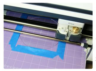
If this happens before engraving, it can also be helpful to watch it trace the acrylic shape. If it traces it perfectly then you know your design is lined up correctly in the program. If it doesn't, you can cancel the cut on your machine and adjust it in the program as needed.
