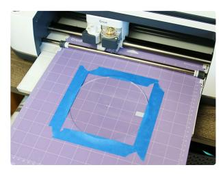
Once the acrylic is securely in place, the design is ready in the cutting program, and the wheels on the roller bar are moved out of place, load the mat into the machine.
