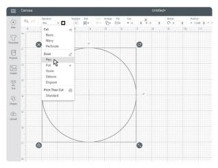
After your shape is made, set it as "draw pen" (or the equivalent on your machine's brand) to keep it separate from the actual engraved design. When we run the actual design later, we will run it without a drawing tool in the machine. This way it will go through the motion, but not touch or write on the acrylic piece.
