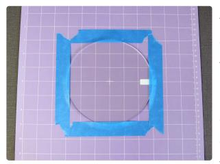
For best results, use painter's tape to hold down the edges of the acrylic as well. This adds an extra layer of security to prevent the acrylic from shifting.
