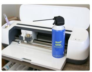
Canned air can also be used to remove the acrylic bits and debris from your cutting machine. Just be very careful what directly you're spraying the air. Don't spray the debris into the inner working of the machine. Instead, be sure to spray them out the front or back openings. Then, sweep up the acrylic pieces with a small broom.
