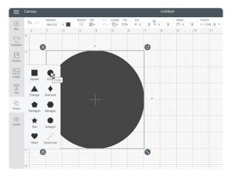
Set the mat aside on a flat surface while you prepare the file in your cutting software. To help line up the design in the software, we will first create the shape of the acrylic. Measure your acrylic, and make a shape as close to your acrylic piece as possible. For example ours is a circle with a 6in diameter.
