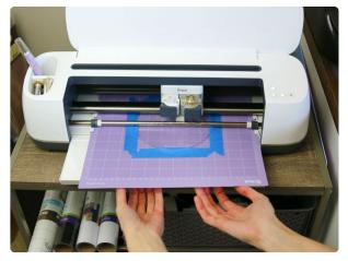
Acrylic is a lot stiffer than the mat, so it is very important to make sure the mat stays flat the entire time it is loaded into the machine and cutting.
