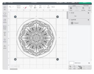
Then attach the shape and the design together in the program. When attached, you want the shape and the design to remain two different objects (I drawing and the other engraving), but have them stuck together how you positioned them (so they do not reorganize and separate when the machine puts them on the mat to start crafting). In Cricut this is called "attach" but it may be called something else in different programs.
