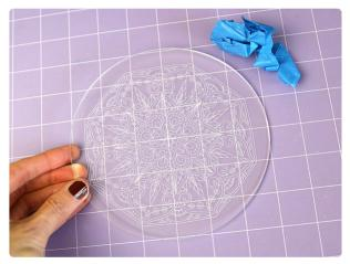
Once the engraving is complete, remove the tape and acrylic from the mat. Be careful not to get fingerprints not the acrylic if possible. Then also remove the protective film off of the back side of the acrylic piece.
