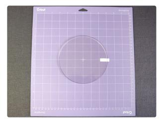
Using the grid, roughly center your acrylic piece on your cutting mat with the engraving side facing up. Paying attention to how the acrylic piece lines up on the grid is very important. This grid will be how we line up our design in the program to make sure it engraves in the correct place.
