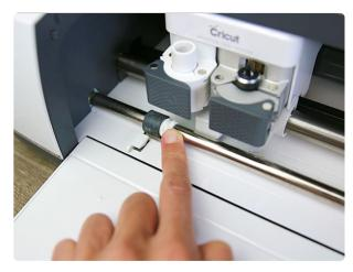
Most cutting machines have small, textured rings on their roller bars. These typically help the roller bar hold onto the mat and move it though the machine.
